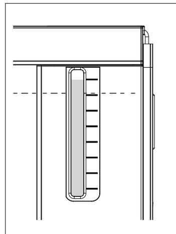
**NOTE:** It is advisable to do the first fill with fresh water or a weak saltwater solution to check the integrity of the system and to clear away any chemical residues from production.
