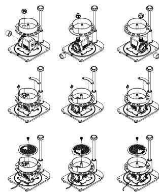
With all of the internal components assembled, lower the skimmer body onto the base so that the hole on the side is aligned with the pump inlet. Secure the body in position tightly with the 4 screws provided.
