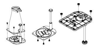
Skimmer Regulator - Rotating the regulator in the "Minus" direction will increase the opening in the base, lowering the foaming point or to produce a drier foam. Rotating in the "Plus" direction decreases the opening in the base, raising the foaming point or to produce a wetter foam.
