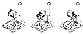
Remove the cable restraint from the base. Run the pump cable around the pump and insert it through the cable channel and under the base. Push the cable restraint back into position.
