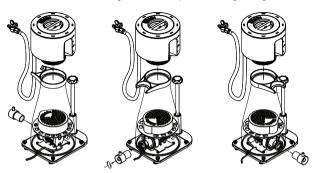
Unscrew the skimmer body from the base and if necessary reposition the pump holder to suit the desired orientation of the pump inlet. Turn the skimmer base upside-down and push the rubber feet firmly into position.
